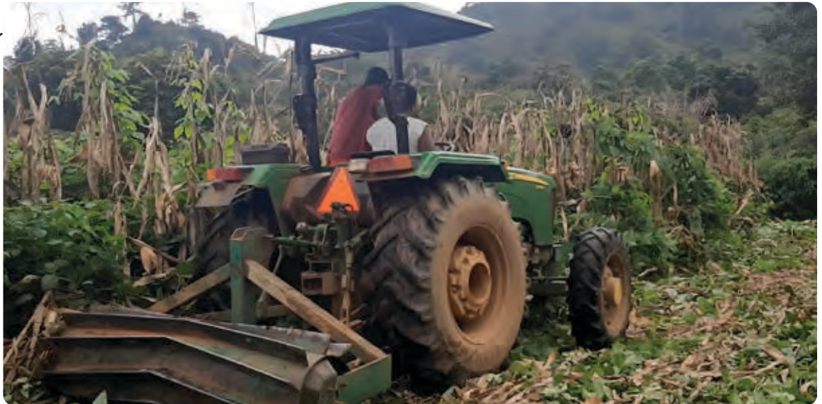
Figure 28: A tractor crimper incorporating climbing beans as green manure before sowing the main crop.
